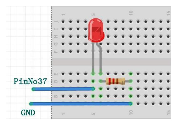
You can refer to this picture to make your circuit on the breadboard. Don't forget that PinNo37 is located on the SERVO1 Interface GPIO port. The GND is located on the SERVO1 Interface as well on the GND port.
