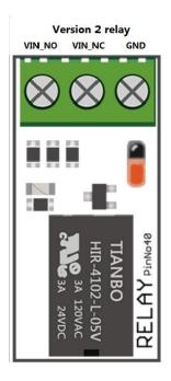
There are two version of Relay in our CrowPi, you can distinguish the version of your CrowPi by the pin name on the relay. Version 1 relay: The names of the three pins on the relay are NO, NC, COM. Version 2 relay: The names of the three pins on the relay are VIN\_NC, VIN\_NO, GND. Note: The method used by different versions of the relay will be different, please choose the method corresponding to your own relay version is to use the relay, otherwise the board may be burned out!
