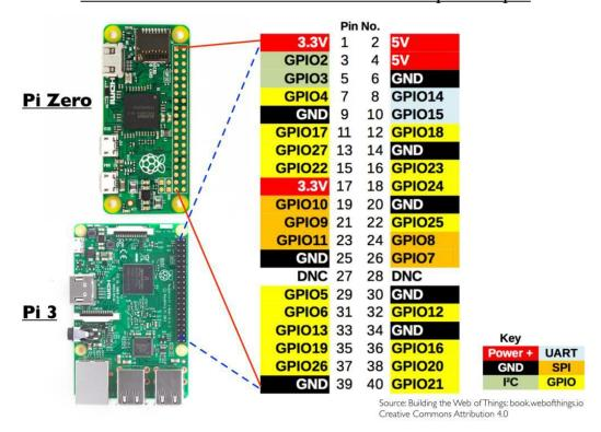
In this lesson we'll go through understanding what GPIO is, how it works and how to control it.
