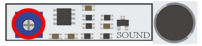
We'll need to turn the little blue square that is circled with a red oval in the picture to either left or right in order to control its sensitivity.
