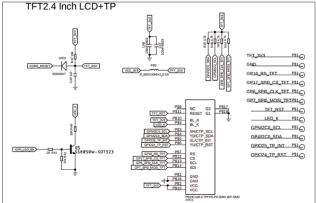
After starting the course, the TFT will display "Please Open the Door." When you press the touch button, the relay will close the circuit (open the door), the relay indicator light will turn on, and the TFT will display a welcome message "Welcome." After a 10-second delay, the relay will automatically open the circuit (close the door), the relay indicator light will turn off, and the TFT will display "Please Open the Door" again.
