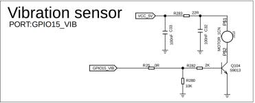
After starting the course, you will observe that as the distance measured by the ultrasonic module changes, the vibration motor will activate when the distance is less than 30 centimeters, indicating that an obstacle has been detected. If the distance reaches or exceeds 30 centimeters, the vibration motor will turn off, indicating that the path is clear and there are no obstacles. If this process does not occur as described, please check whether the program is running correctly.
