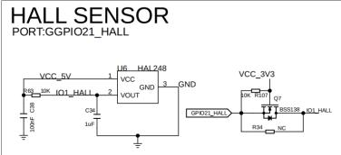
After starting the course, the TFT will display "Counter: 0." Each time you bring a magnet close to the Hall sensor, the red light will turn on once, and the TFT will display the count incremented by 1, and so on.
