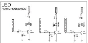
After starting the course, when the ambient light is very strong, the LED will not turn on regardless of whether there is any sound. When the ambient light is very dim or when the light sensor is covered by hand, the LED will remain off by default. At this time, if a sound is detected, the LED will turn on for 10 seconds and then turn off. If sounds are detected continuously, the LED will remain on until there is no sound for 10 seconds, after which it will turn off.
