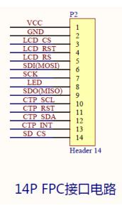
P2 is the module 14P FPC cable interface, which can only be connected to
