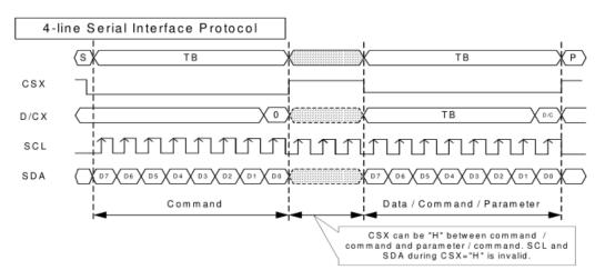
CSX is a slave chip selection, and the chip will only be enabled when CSX is at low
