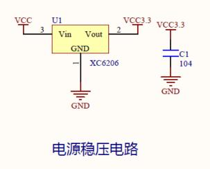
This circuit is used to stabilize the input voltage of the module, where VCC is the external input voltage, VCC3.3V is the module input voltage, and C1 is the bypass filter capacitor. VCC can be connected to 5V or 3.3V, and it is recommended to connect to 5V because only by connecting to 5V can VCC3.3 output 3.3V. If connected to 3.3V, VCC3.3 output voltage will be less than 3.3V, which will cause the backlight brightness of the LCD screen to darken.
