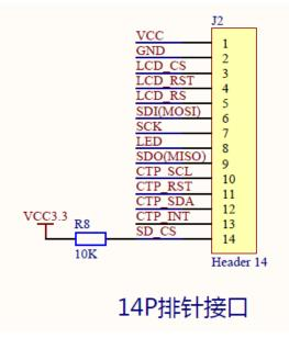
J2 is 14P pin, R8 is the pull-up resistor of SD card CS pin. The 14P pin is used to connect to the main control, which can be directly inserted or connected through a DuPont cable. Because the SD card and LCD share the SPI bus, first pull up the CS pin of the SD card to disable its functions and avoid SPI bus device conflicts when the module is in use.
