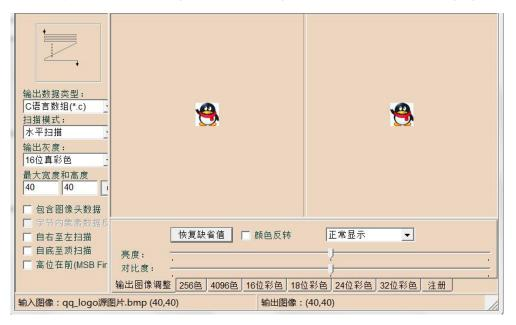
The Image2Lcd software needs to be set to scan horizontally, from left to right,
