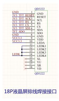
QD3222 is a 18P pad with a spacing of 0.8mm. Used to weld the LCD so that it can receive signals from the main control.
