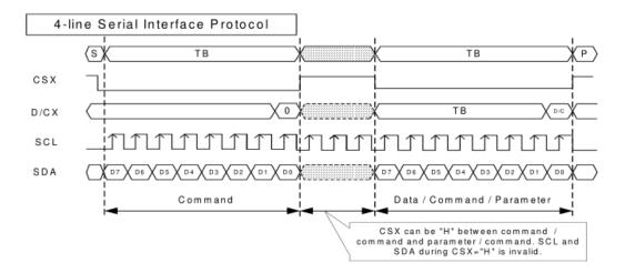
CSX is a slave chip selection, and the chip will only be enabled when CSX is at low power level.
