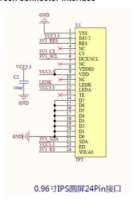
U1 is a 24P narrow spacing (0.4mm) double row connector base. It is used to connect to the FPC cable of the LCD, so that the LCD can receive signals from the main control. C2 is the bypass filter capacitor of the LCD power supply.
