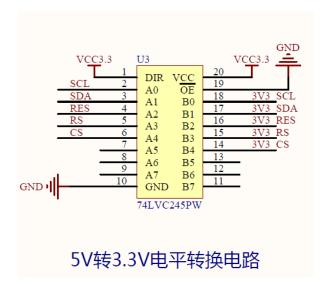
U3 is a level conversion IC that converts between 5V and 3.3V. This circuit only uses the unidirectional function of 5V to 3.3V, and the 5V or 3.3V level signals input by the main control are converted through this circuit and then output to the LCD screen.
