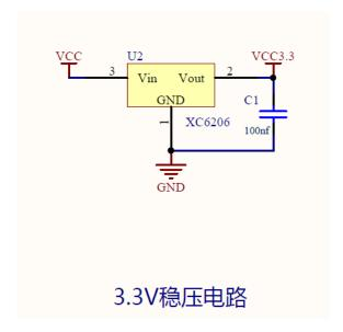
This circuit is used to stabilize the input voltage of the module, where VCC is the external input voltage, VCC3.3V is the module input voltage, and C1 is the bypass filter capacitor. VCC can be connected to 5V or 3.3V, and it is recommended to connect to 5V because only by connecting to 5V can VCC3.3 output 3.3V. If connected to 3.3V, VCC3.3 output voltage will be less than 3.3V, which will cause the backlight brightness of the LCD screen to darken.
