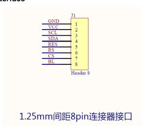
J1 is an 8P slot interface that requires a DuPont cable with a 1.25mm spacing and connectors to be connected.
