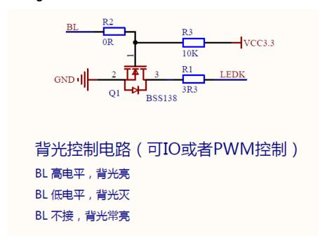
R2 is reserved for compatibility with J3Y control circuits, directly using a 0 ohm resistor. R1 is the backlight current limiting resistor, R3 is the pull-up resistor,
