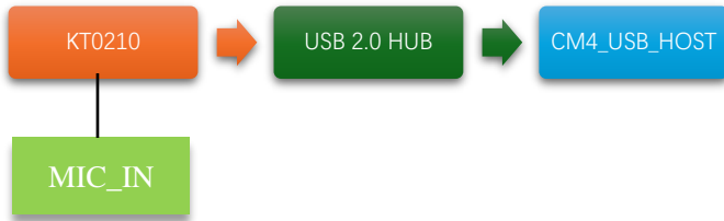
Figure 7:USB interface hardware connection diagram
